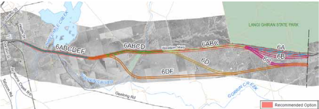
Figure 17: Shortlisted alignment options between Langi Ghiran and Ararat
